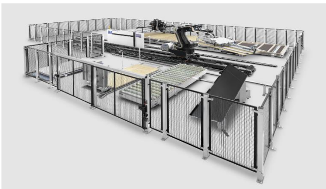
Figure 8: Highly efficient production in timber construction with robots and multifunction bridges
