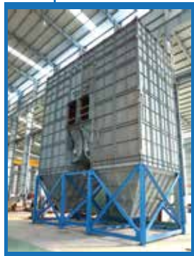
Bag Filter (Fine Filter) Filtration efficiency up to 99%
